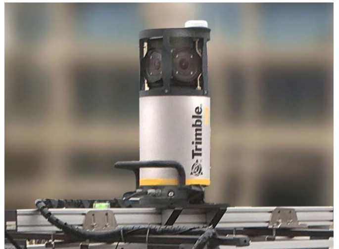
The Trimble MX7 collects 360-degree images and IMU/GNSS data from a moving platform.
